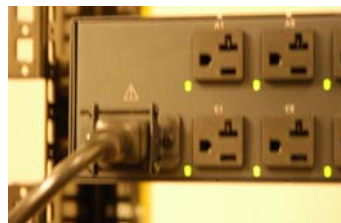
Removable power cables look like this. These types of power cables are secured in place with a bracket that is included on the SPC models with removable power cables.
