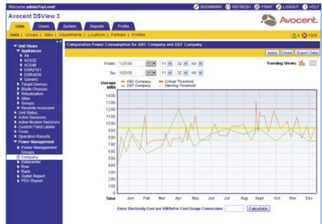
Comparative Power Consumption Report (by Racks, Rows, Data Center, or Companies)
