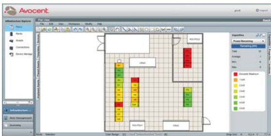
In this top-down view, a rack displayed in red indicates it's exceeding a pre-defined power capacity policy.
